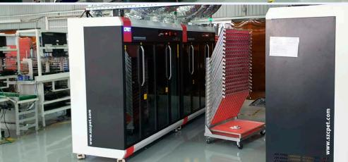
A fully automated line for surface mounting of electronic modules on printed circuit boards (SMT technology) has been installed, adjusted and launched at the Kvant plant.
