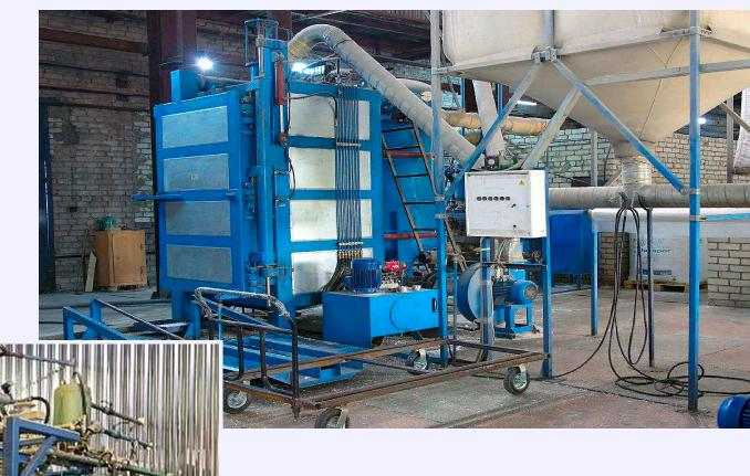
The workshop is equipped with three KURTZ K 14.5 12S/F molding machines (Shuttle EPS), Atmos ST 90 compressor station and UPE-600 steam generator.
